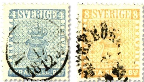
Parts of the print is missing, due to inadequate adjustment of the level of the printing blocks.
